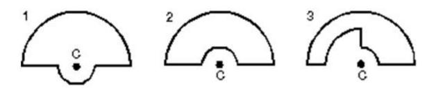
**Sample Question:** Consider the long cylindrical conductor with the cross section shown below, which carries a current I uniformly distributed across the area of the conductor, and going into the page.
