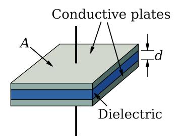
**Sample Question:** Consider a parallel-plate air-gap capacitor with charge q and plate area A.
