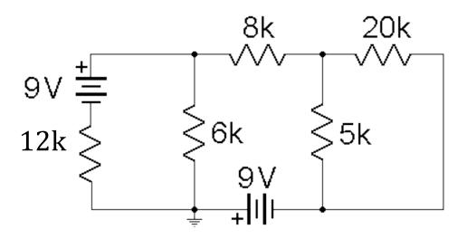
A. Simplify the right portion of the circuit as much as possible, by using series and parallel equivalent resistances, and draw the simplified equivalent circuit
